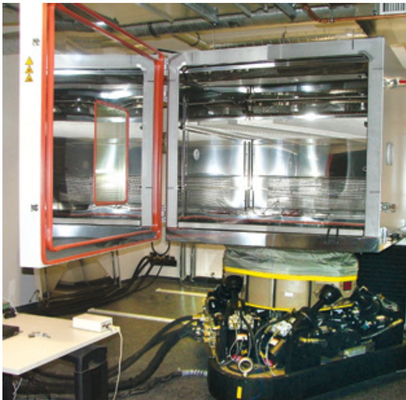
Model 353 MAST system with integrated environmental chamber at PLDS Automotive Test Laboratory in Wetzlar Germany (Photo courtesy of PLDS Germany GmbH)
